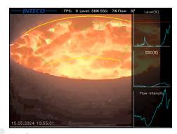
The IRVA-VD transforms any existing camera into a powerful tool for monitoring and optimizing vacuum tank degassing processes. The algorithm evaluates the effectiveness of gas stirring, the exposed stirring eye and the critical slag foaming events through real-time video analysis. This contributes to proactive process management and further improves the accuracy of degassing models.
